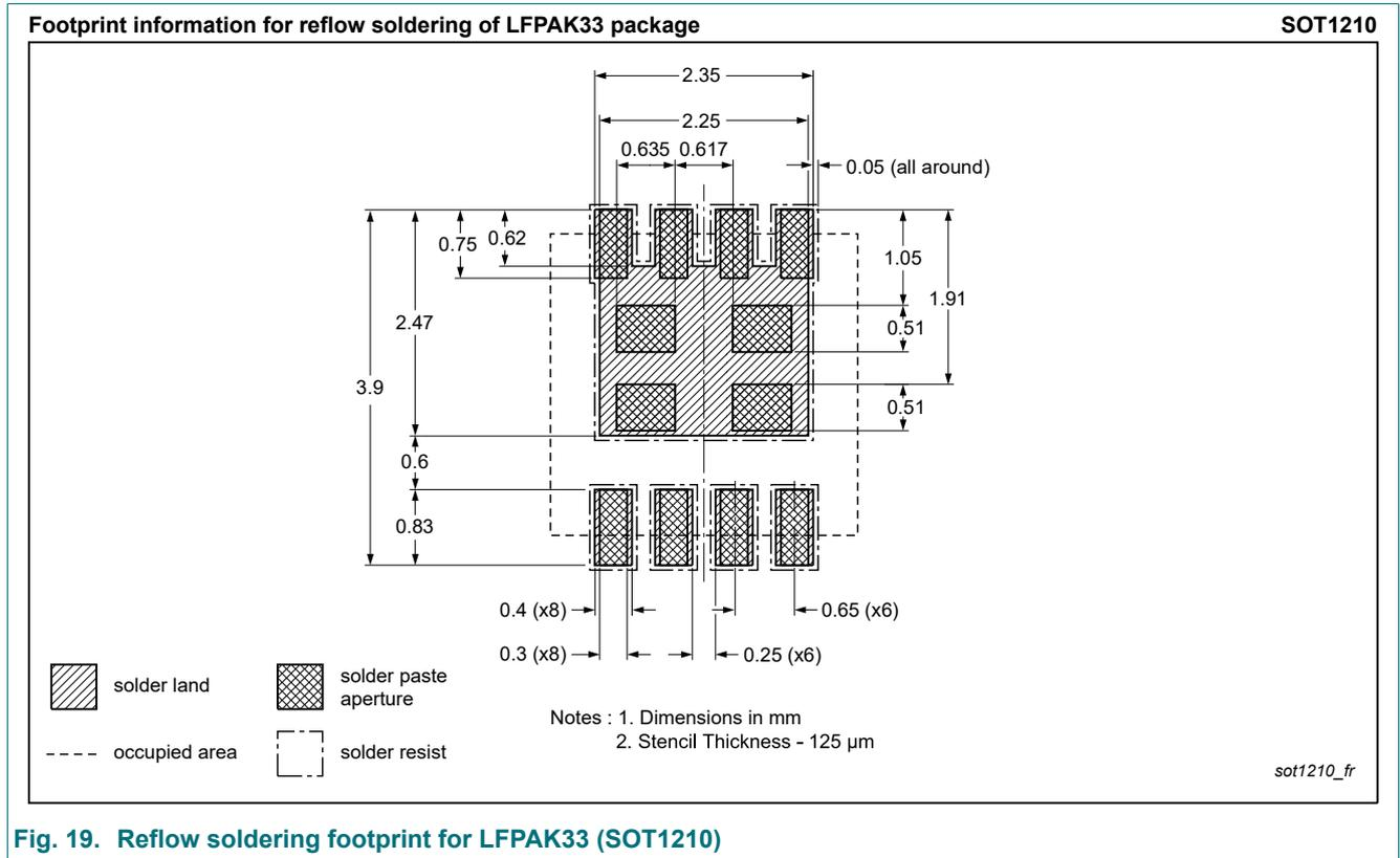
**Fig. 19. Reflow soldering footprint for LFPAK33 (SOT1210)**
