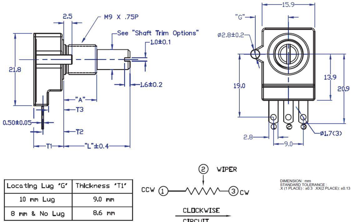
Series 282S Metal Shaft, Bushing Mount, Solder Lug "S" Type Terminal Formed to Rear
