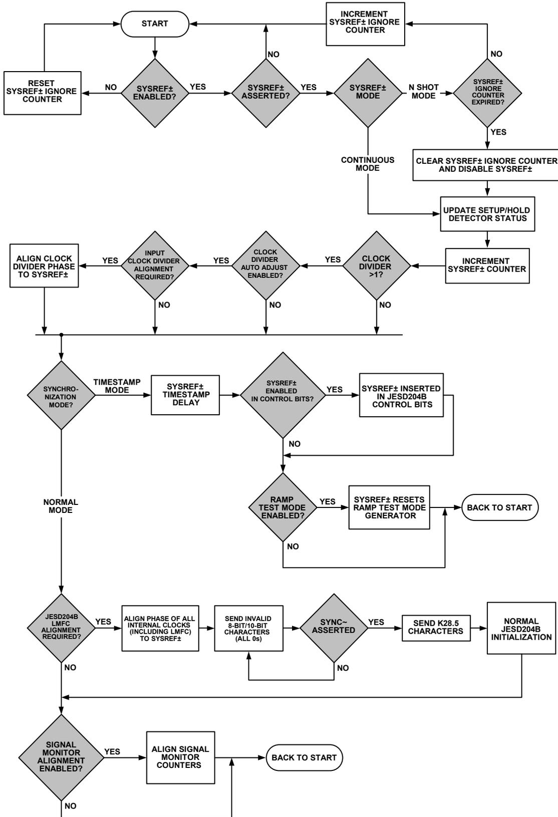
Figure 74. SYSREF± Capture Scenarios and Multichip Synchronization
