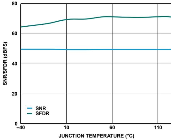
Figure 18. SNR/SFDR vs. Junction Temperature,  $f_{IN} = 611$  MHz
