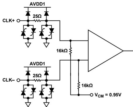
Figure 33. Clock Inputs
