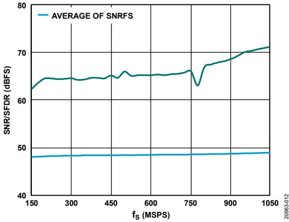
Figure 12. SNR/SFDR vs. Sample Rate ( $f_s$ ),  $f_{IN} = 155$  MHz
