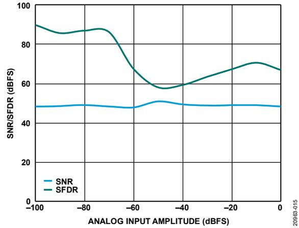
Figure 15. SNR/SFDR vs. Analog Input Amplitude,  $f_{IN} = 155$  MHz
