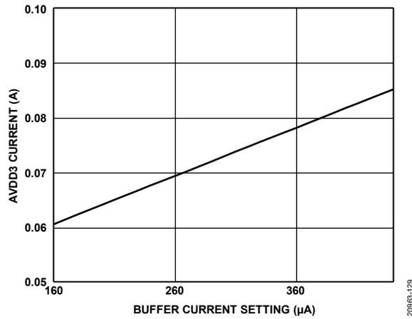
Figure 30. AVDD3 Current vs. Buffer Current Setting
