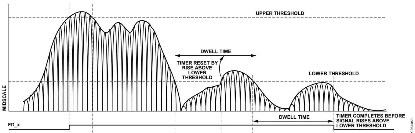
Figure 55. Threshold Settings for the FD\_x Signals
