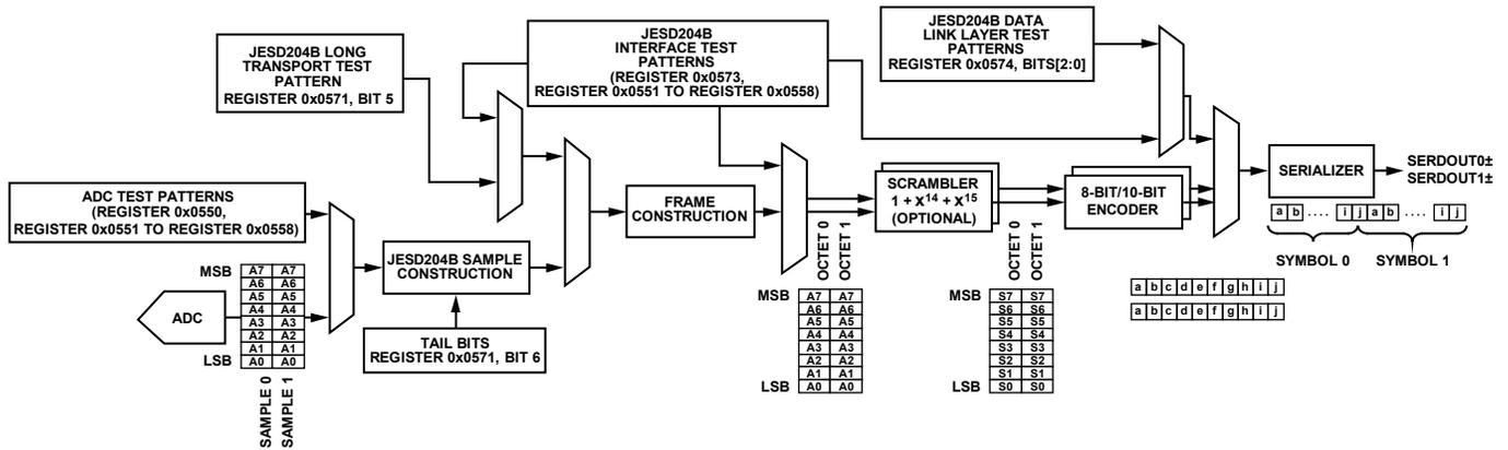
Figure 61. ADC Output Datapath with Data Framing
