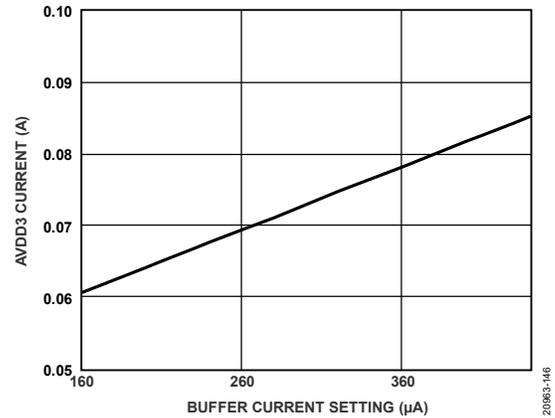
Figure 46. AVDD3 Power vs. Buffer Current Setting
