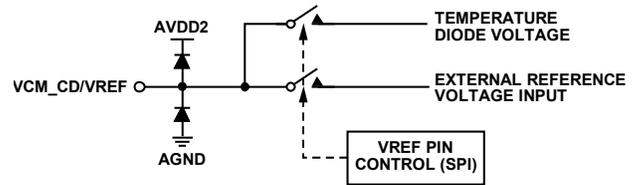
Figure 42. VCM\_CD/VREF Input/Output
