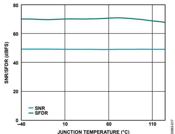
Figure 17. SNR/SFDR vs. Junction Temperature,  $f_{IN} = 155$  MHz
