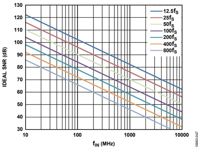
Figure 52. Ideal SNR vs.  $f_{IN}$  over Jitter
