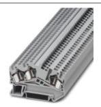
Feed-through terminal block, Connection method: Spring-cage connection, Cross section: 0.08 mm² - 6 mm², AWG: 28 - 10, Width: 6.2 mm, Color: orange, Mounting type: NS 35/7,5, NS 35/15
