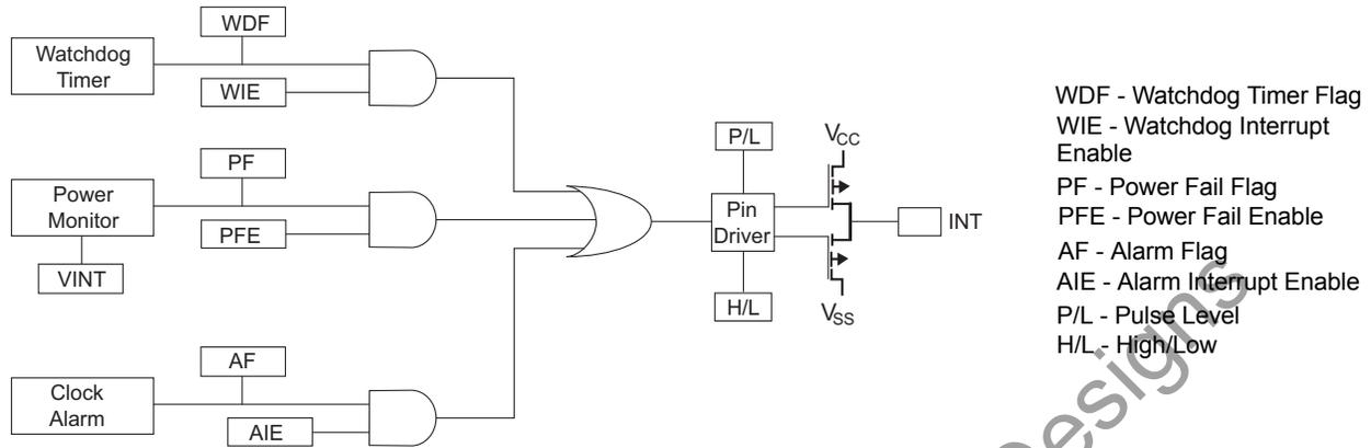
Figure 6. RTC Recommended Component Configuration
