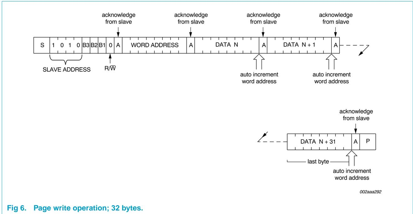
Fig 6. Page write operation; 32 bytes.
