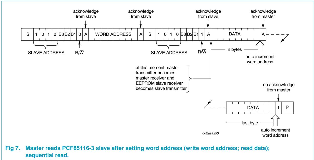
**Fig 7. Master reads PCF85116-3 slave after setting word address (write word address; read data); sequential read.**
