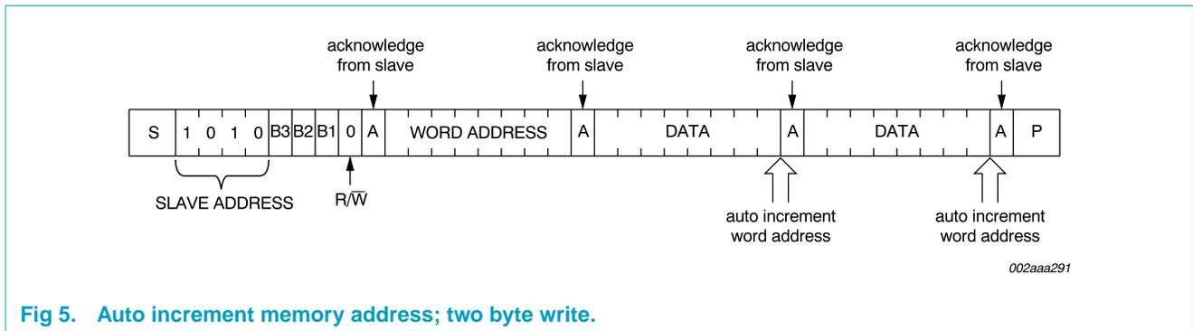
Fig 5. Auto increment memory address; two byte write.
