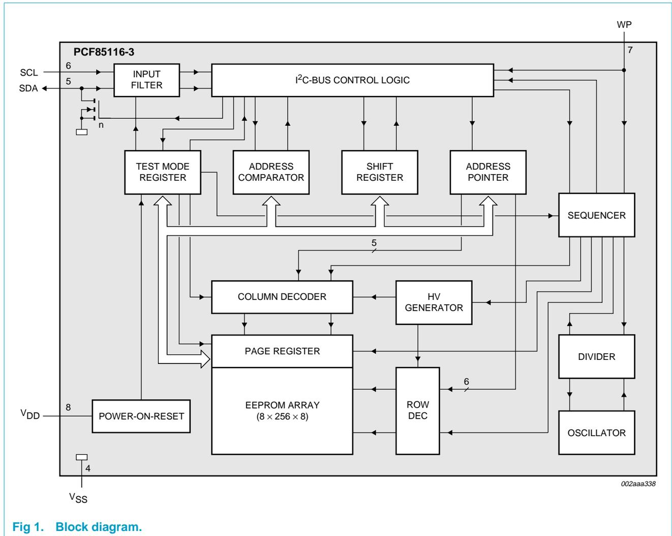
Fig 1. Block diagram.
