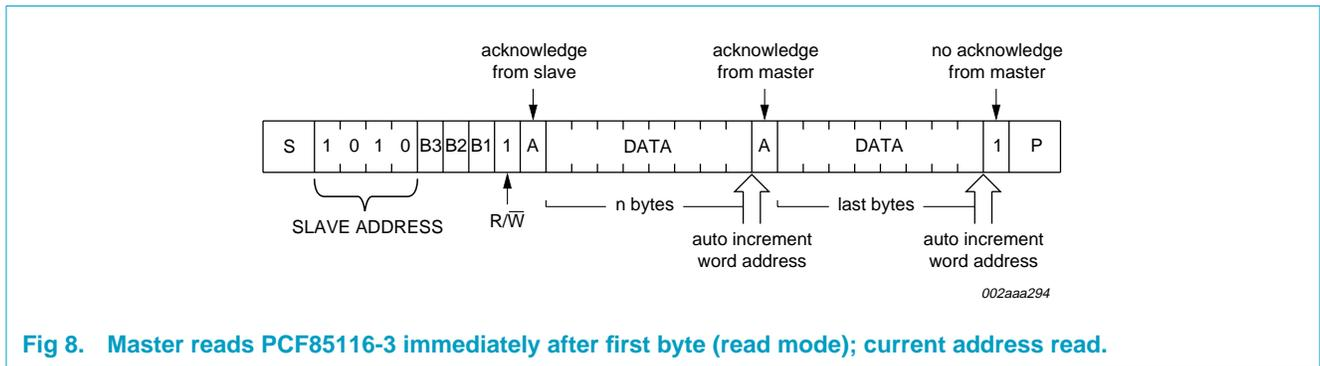
**Fig 8. Master reads PCF85116-3 immediately after first byte (read mode); current address read.**
