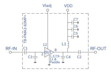
Fig 1. Application and Characterization Circuit
