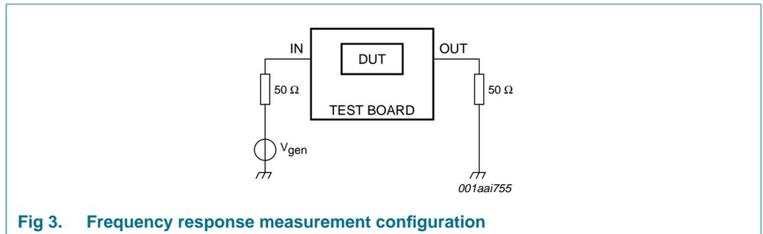
**Fig 3. Frequency response measurement configuration**
