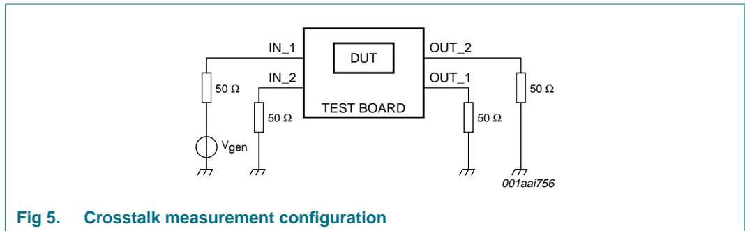
The crosstalk between adjacent channels within the IP3337CX18 for different channel pairs measured in a 50 Ω NetWork Analyzer (NWA) system, is shown in [Figure 6](#). In all cases, all unused connections are terminated with 50 Ω to ground.
