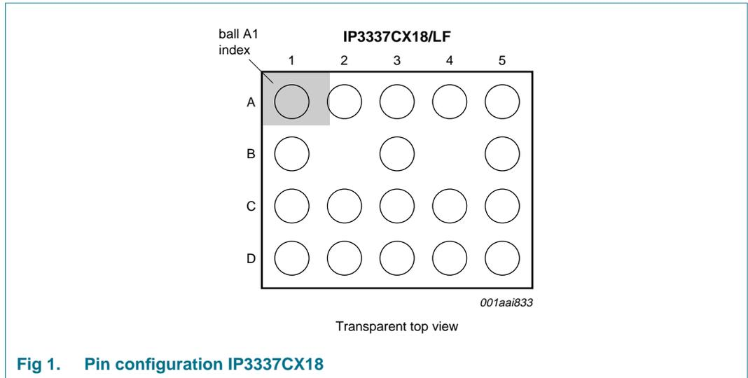
Fig 1. Pin configuration IP3337CX18
