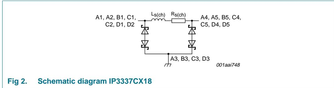
Fig 2. Schematic diagram IP3337CX18
