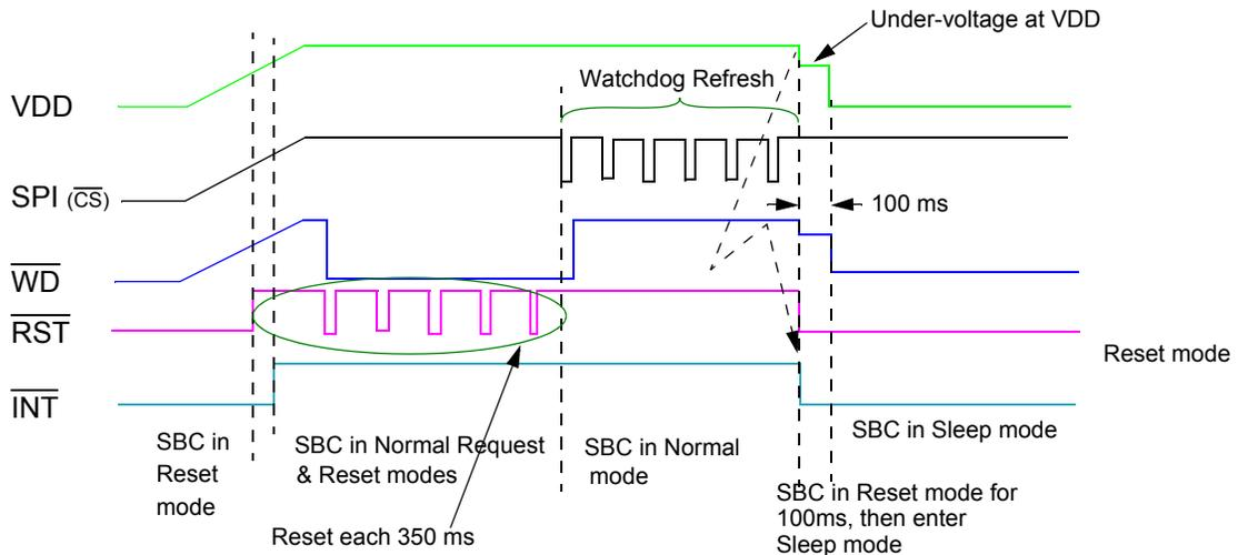
**Figure 35. Under-voltage at VDD. Sleep mode selected.**
