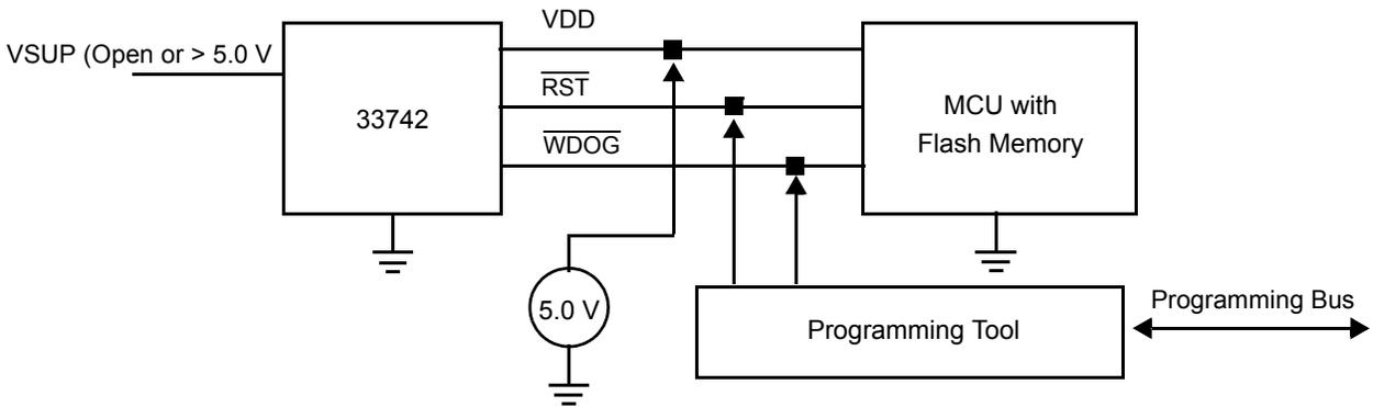
**Note** External supply and sources applied to VDD,  $\overline{\text{RST}}$ , and  $\overline{\text{WDOG}}$  test points on application circuit board.
