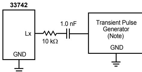
Note Waveform per ISO 7637-1. Test Pulses 1, 2, 3a, and 3b.
