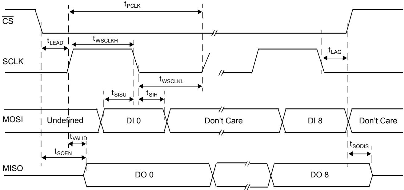
**Note** Incoming data at MOSI pin is sampled by the 33742 at SCLK falling edge. Outgoing data at MISO pin is set by the 33742 at SCLK rising edge (after  $t_{VALID}$  delay time).
