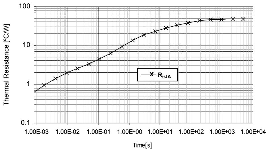
**Figure 41. Transient Thermal Resistance  $R_{\theta JA}$ ,
