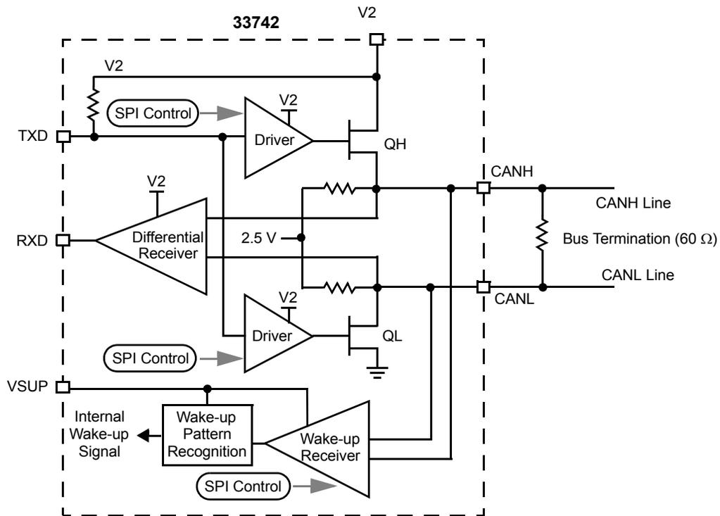
**Figure 19. Simplified Block Diagram of CAN Interface**
