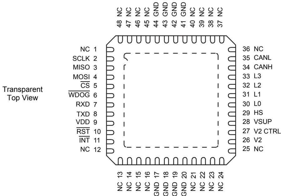
**Figure 4. 33742 48-Pin Connections**
