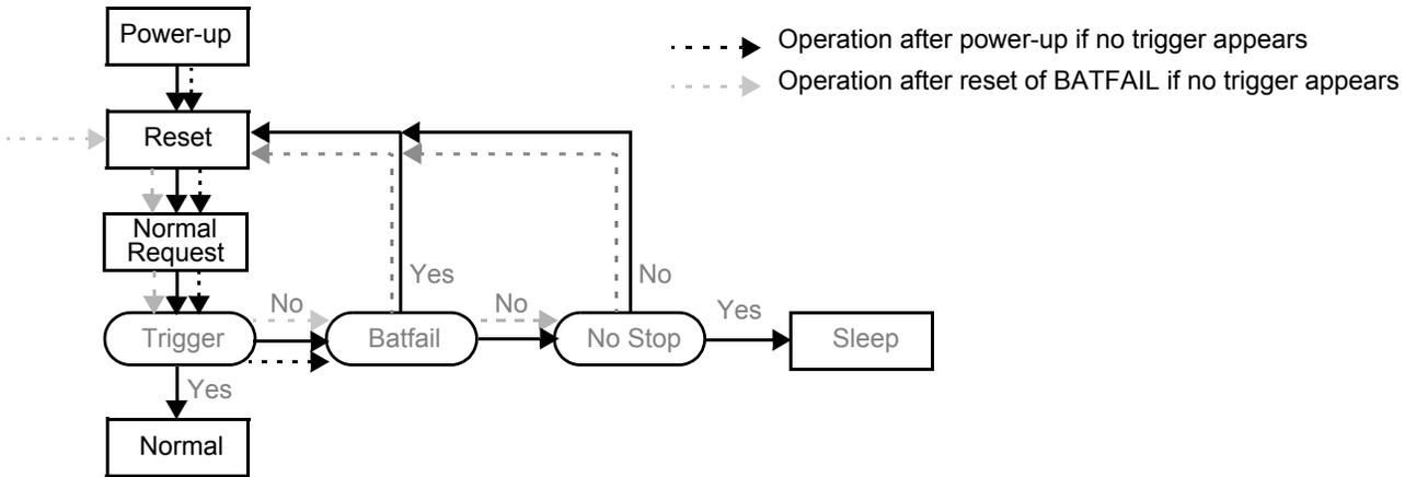
**Figure 14. Operation After SBC Power-up**
