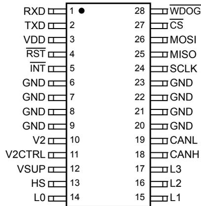
**Figure 3. 33742 28-Pin Connections**
