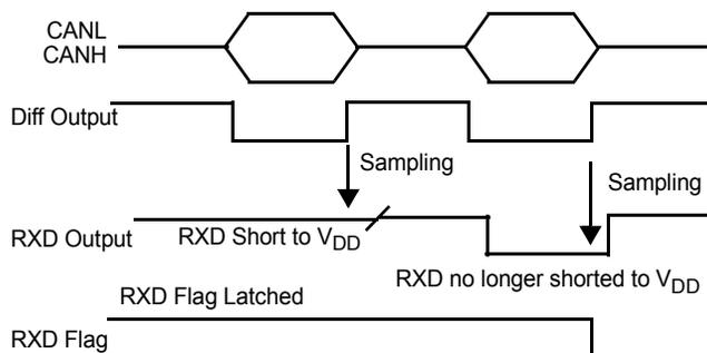
**Note** RXD Flag is neither the RXPR bit in the LPC register nor the CANF bit in INTR register.
