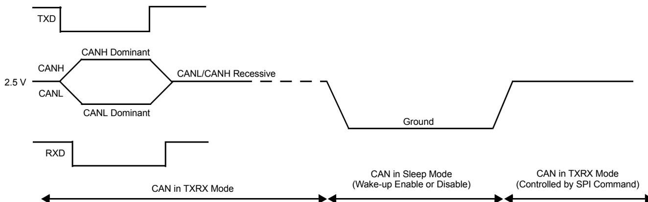
Figure 21. CAN Signals in TXRX and Sleep Modes
