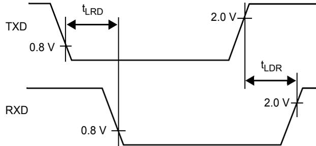
**Figure 8. Propagation Loop Delay TXD to RXD**
