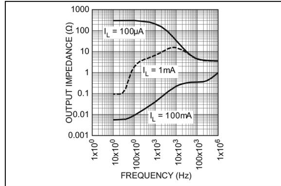
**FIGURE 2-22:** Output Impedance.
