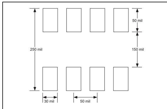
**FIGURE 4-4:** Minimum Recommended SOIC-8 PCB Pads Size.
