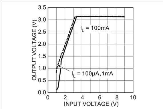
**FIGURE 2-3:** Dropout Characteristics.
