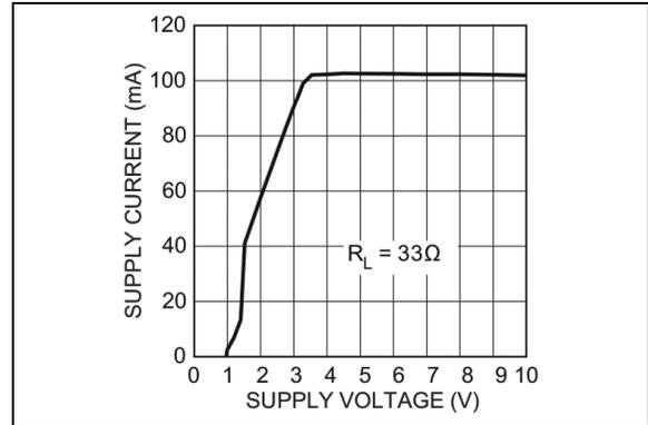
**FIGURE 2-16:** Supply Current vs. Supply Voltage (3.3V Version).
