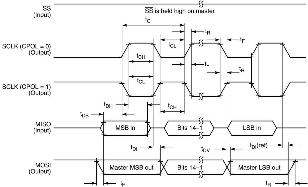
Figure 14. SPI master timing (CPHA = 0)
