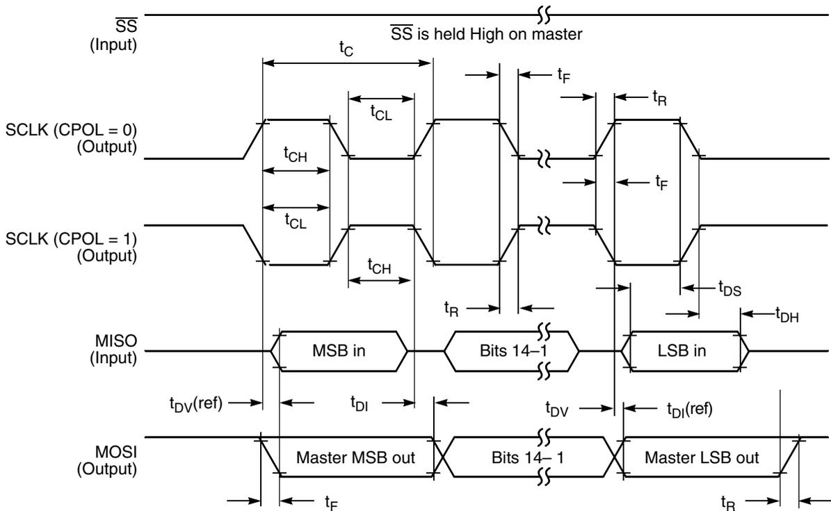
Figure 15. SPI master timing (CPHA = 1)
