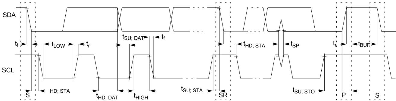
Figure 21. Timing definition for fast and standard mode devices on the I<sup>2</sup>C bus
