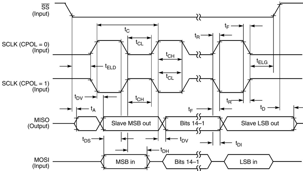
**Figure 17. SPI slave timing (CPHA = 1)**
