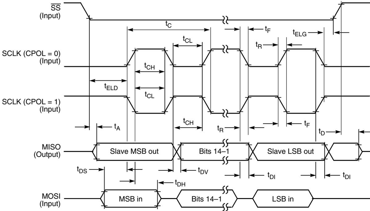
**Figure 16. SPI slave timing (CPHA = 0)**
