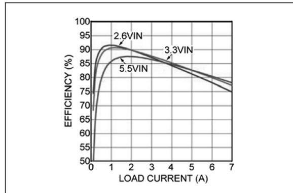
**FIGURE 2-12:** Efficiency at  $1.2V_{OUT}$ .
