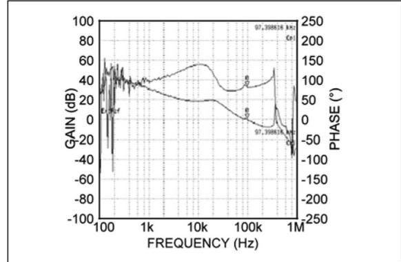
**FIGURE 2-16:** Bode Plot ( $V_{IN} = 5.5V$ ,  $V_{OUT} = 1.8V$ ).
