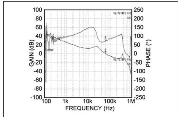
**FIGURE 2-17:** Bode Plot ( $V_{IN} = 5.0V$ ,  $V_{OUT} = 3.3V$ ).
