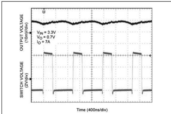
**FIGURE 2-21:** Switching Waveforms.
