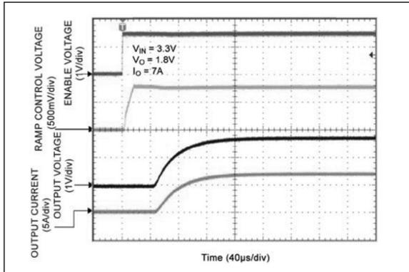
**FIGURE 2-19:** Start-Up ( $C_{RC} = 0\text{ nF}$ ).
