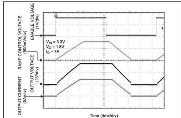
**FIGURE 2-18:** Start-Up/Shutdown ( $C_{RC} = 10\text{ nF}$ ).
