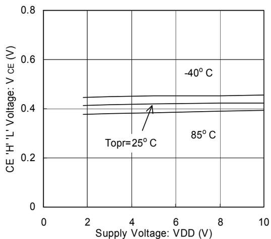
(9) PWM 'H' 'L' Voltage vs. Supply Voltage
