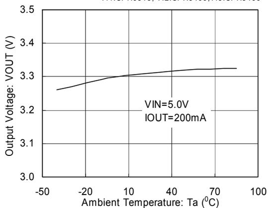
(17) Output Voltage vs. Ambient Temperature 2
